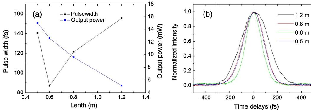
**Fig. 3** (a) The output power (blue square) and the corresponding pulse width (black square) of the 1150-nm femtosecond sources. (b) Autocorrelation traces of the 1150-nm femtosecond sources, which is generated by the SHG of 2300-nm solitons from a different length of fibers.
