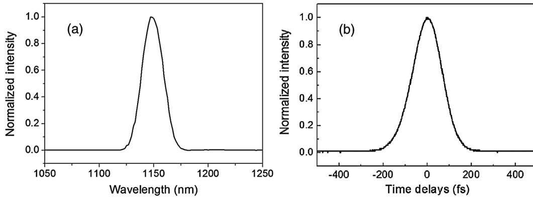
**Fig. 5** The (a) spectra and (b) autocorrelation trace of the SHG signals from MgO:PPLN.
