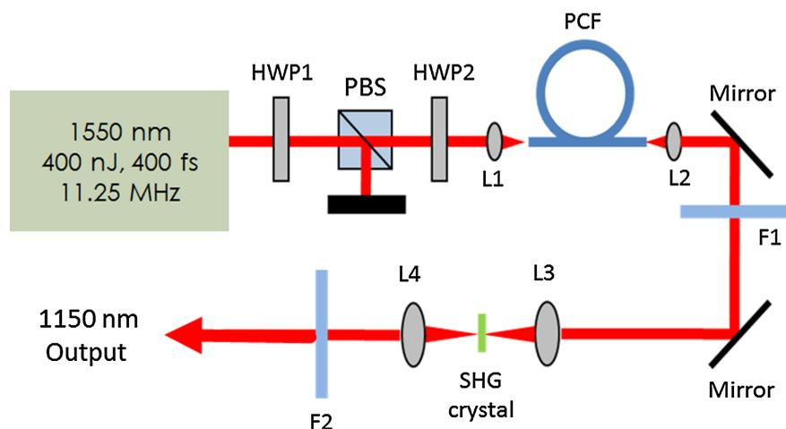
**Fig. 1** Schematic diagram of the 1150-nm laser system. HWP, half-wave plate; PBS, polarization beam splitter; PCF, photonic crystal fiber; L, lens; F, filter; SHG, second harmonic generation.
