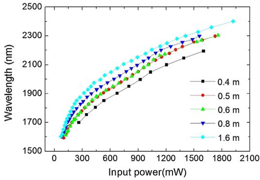
**Fig. 2** The relation between the wavelength of fundamental soliton and input power for difference length fibers.
