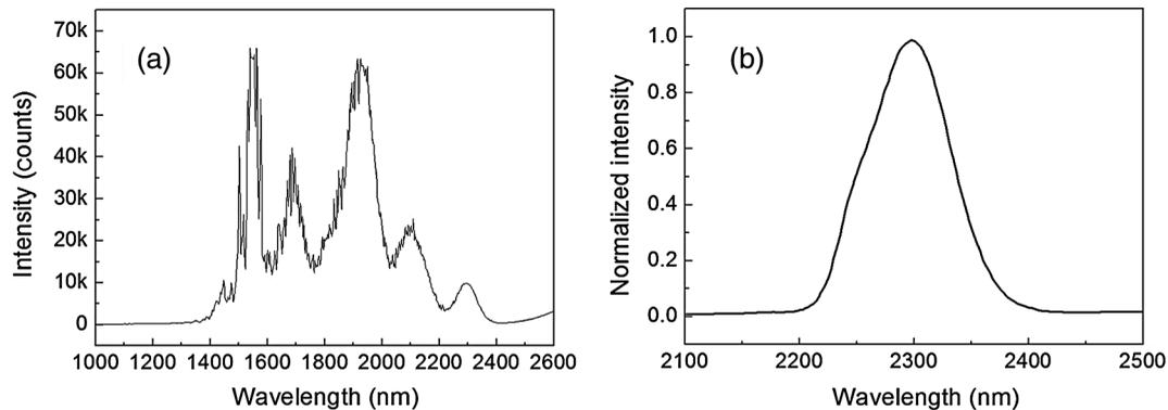
**Fig. 4** The spectra of (a) solitons in a 0.6-m photonic crystal fiber. (b) The 2300-nm soliton spectrum after passing the 2250-nm long pass filter.
