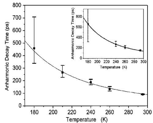
FIG. 2. Anharmonic decay time (solid squares) of 470 and 380 GHz (inset) longitudinal coherent acoustic phonons propagating in GaN at different temperatures. Error bars represent the standard deviation of measured values. Described by Eq. (2) (solid curve), the decay time shows an inverse cubic dependence on temperature.
