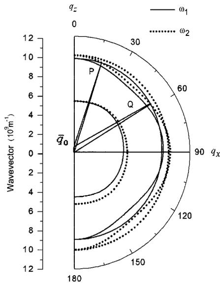
FIG. 3. Conservation surfaces of  $\omega_1$  (solid curve) and  $\omega_2$  (dotted curve) with the origin of the  $\omega_1$  surfaces moved by the wave vector of LA phonons. Point  $P$  is related to the occasional intersection close to the  $q_z$  direction and point  $Q$  is related to the nearly occasional intersection close to the  $q_x$  axis.
