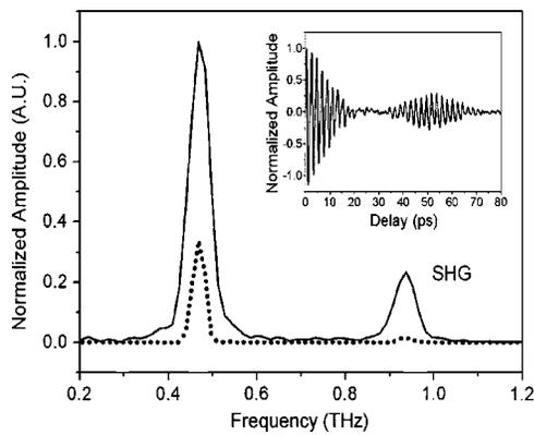
FIG. 1. Differential transient transmission trace of the studied sample with InGaN/GaN MQW at 80 K (inset) and its corresponding power spectra during the generation (solid curve) and echo (dotted curve) phases.
